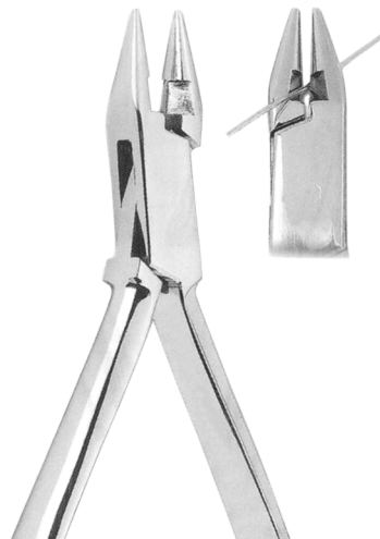
SS-7-5135 Bird beak pliers for bending round, square or rectangular wire up to 0,7 mm. (.028"). With cutter.
